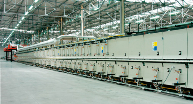
Ceramics industry: roller hearth kiln
